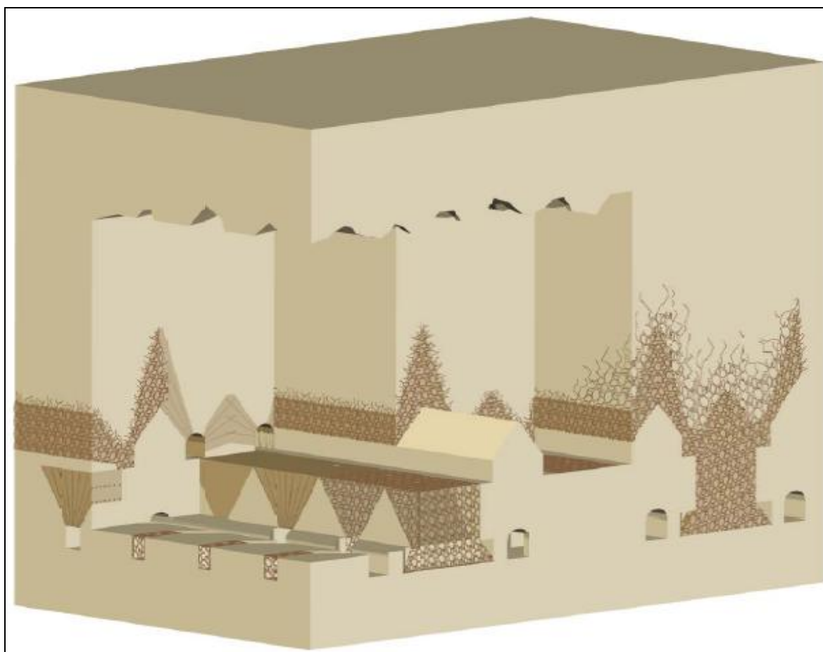
Figure 4.9: Block Cave Schematic
