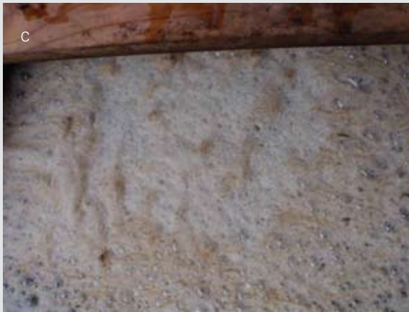
Figure 13. (a) Leading edge of foam in skimmer box showing initial development of brown material on surface; (b) more compressed foam showing larger surface bubbles, and thicker layers of brown flocculated material; (c) white foam exposed when overlying brown material is removed (note bubble size is much smaller in underlying foam); (d) 'coherent' foam created by collection and concentration in skimmer box.
