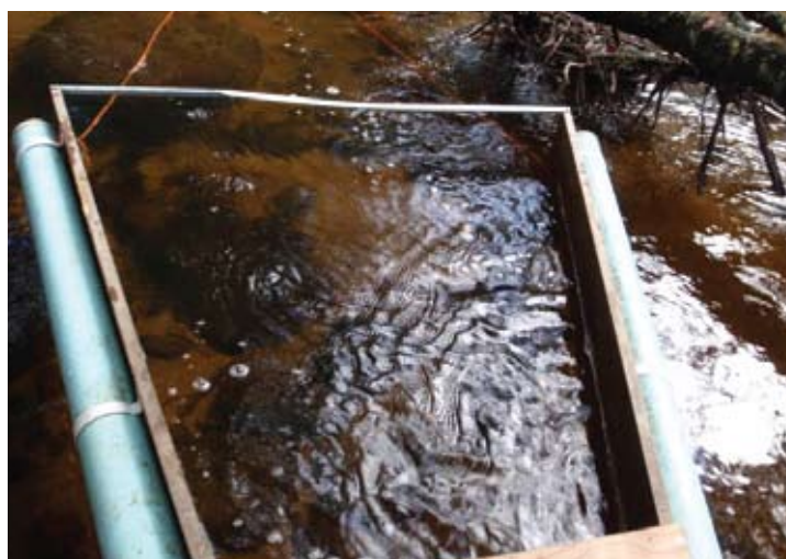
Figure 12. Natural foam in S. George River prior to collection. Opening of skimmer box is approximately 1.25 m.
