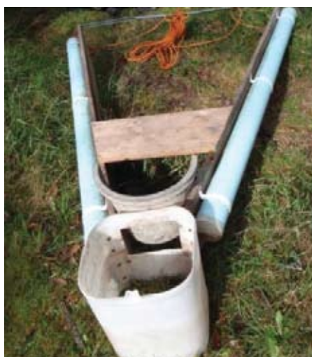
Figure 11. Photo showing the latest skimmer box construction
